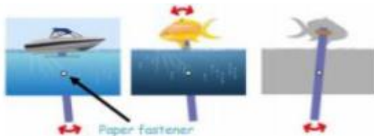
Levers can be used with or without a slot. The fish and boat are glued to the lever which is used as a handle.
